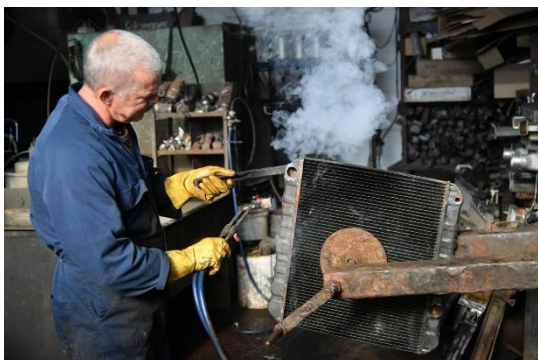
Caption: From cleaning radiators with a bead blaster, to using gas torches for welding - compressed air is an essential utility used and relied upon every day in Trevor French Radiators' workshop.
