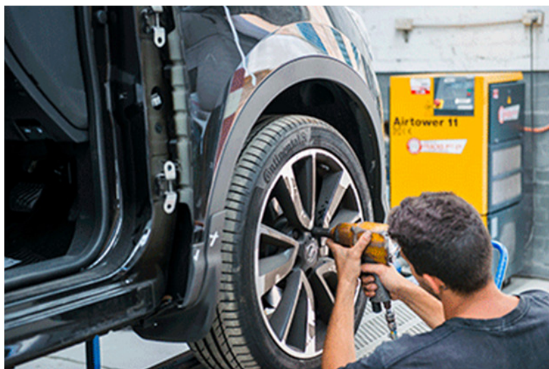
Caption: Compressed air used here to power an air tool at KBW
