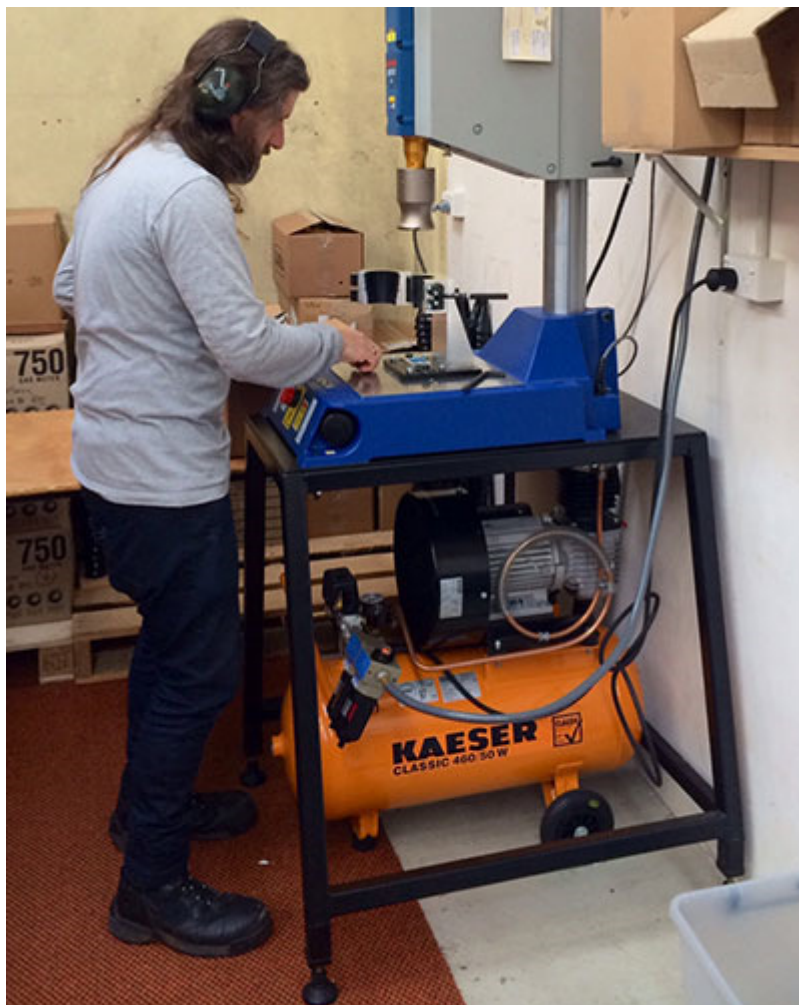
Caption: A Kaeser Classic workshop compressor powers the plastic welder used in the assembly of the sshhmute Practice Mute
