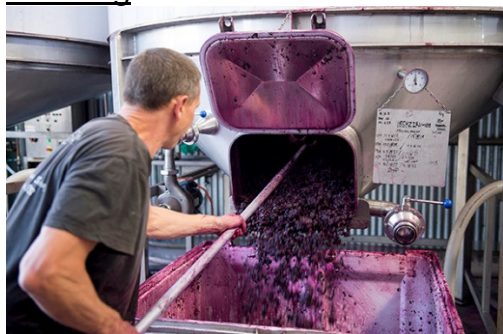
005_Image 8_skins being transferred from fermenters to pneumatic press at Teusner Wines.jpg 005_Image 9_skins being transferred from fermenters to pneumatic press at Teusner Wines 2.jpg
