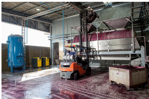
005_Image 10_Pneumatic press being filled at Teusner Wines.jpg 005_Image 11_Pneumatic press being filled at Teusner Wines 2.jpg
