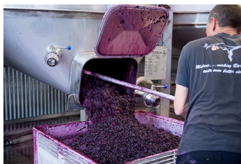
005_Image 8_skins being transferred from fermenters to pneumatic press at Teusner Wines.jpg 005_Image 9_skins being transferred from fermenters to pneumatic press at Teusner Wines 2.jpg
