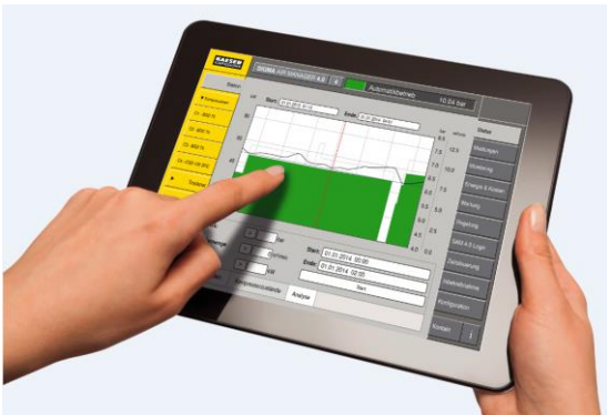
Caption: From a PC, laptop, tablet or smartphone - the SAM 4.0's integrated web server provides a visual display of all compressed air system data in the form of HTML pages.
