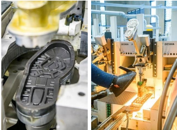
Caption: Representing the latest method of attaching soles to footwear uppers - here the advanced dual density soles of all Mongrel Boots are directly injected onto an upper.
