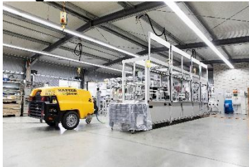
Caption: Mobile compressors are a good solution when compressed air is required quickly. Mobile compressors with an electric drive, can also be set up inside buildings.
