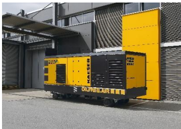
Caption: For large and oil-free compressed air requirements, compressors such as the M 500-2 are available.
