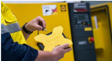
**Caption:** The Air Demand Analysis (ADA) measuring equipment logs a compressed air system for a fixed period of time.
