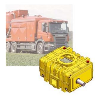
The "Omega PV" rotary blower block is equipped for vacuum operation and features pre-inlet cooling. "PV" blowers can achieve 90 % vacuum and are perfect for a wide variety of applications ranging from pneumatic conveying to vacuum generation in tanker trucks and suction vehicles, as well as in mobile grinding and mixing systems.
