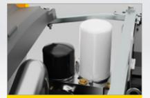
Oil separation with spin-on cartridges
