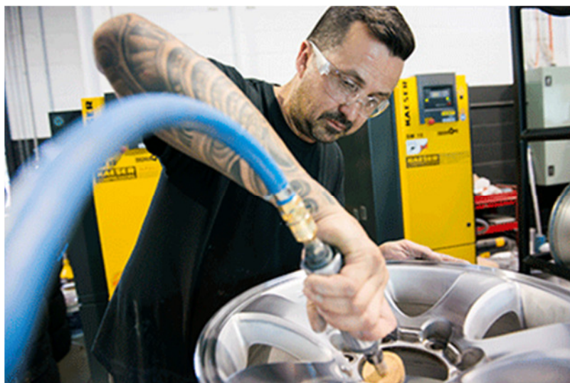
Caption: Compressed air extensively in the repair and refurbishment process; here powering a pneumatic tool
