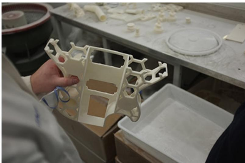
Caption: The SLS printing process involves a laser being aimed into a bed of nylon powder. The laser fuses (or sinters) the nylon powder, layer upon layer. Once cooled, excess powder is then brushed off to reveal the three-dimensional shape
