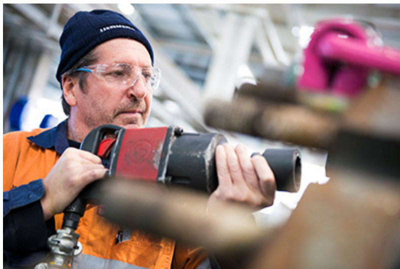
Caption: From the dismantling area to the reassembly area, compressed air is used to power large torque and rattle guns, grit blasting as well as the painting booth
