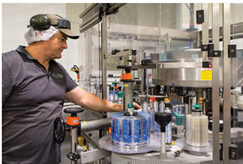
Caption: Compressed air is used to power the labelling machines at E'stel
